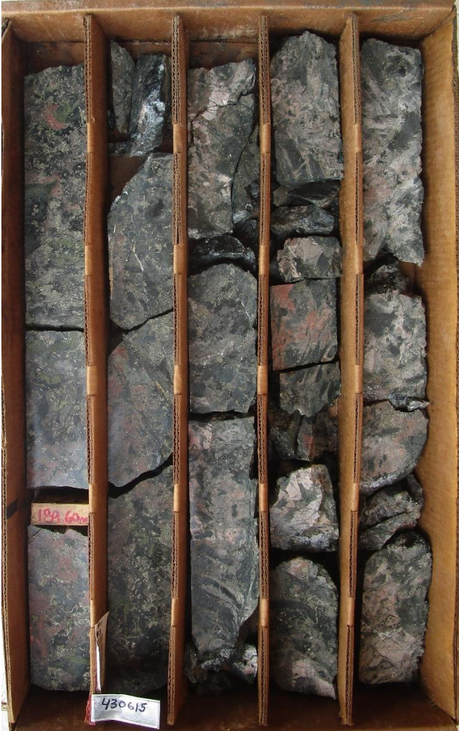
Image 2: Photo of split core from drill hole CC24_001 (189.40m to 192.15m) showing intensely sulfidized and silicic epidote skarn with probable potassium feldspar alteration
