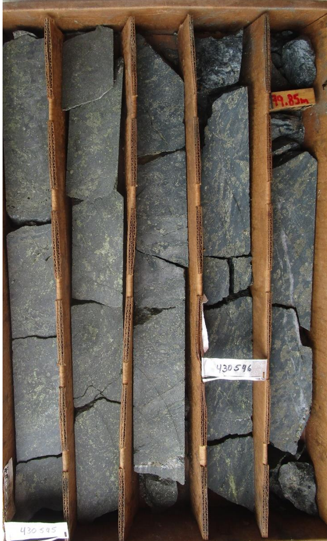
Image 1: Photo of split core from drill hole CC24_001 (77.00m to 79.90m) showing chloritic magnetite skarn with chalcopyrite observed throughout
