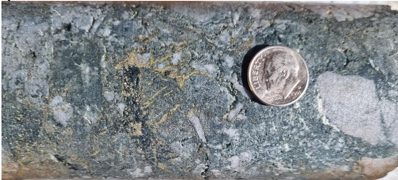
Image 2: Drillhole CC25_037 at 266.7m showing veinlets of chalcopyrite>pyrite in the Courtland Hydrothermal Breccia
