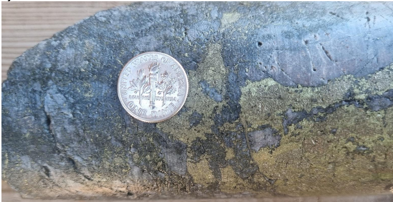
Image 1: Drillhole CC25_037 at 258.2m showing patches of chalcopyrite>pyrite in the Courtland Hydrothermal Breccia
