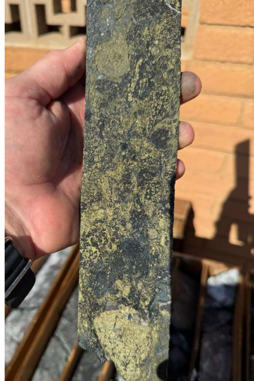
High-grade replacement style massive sulphide mineralization intercepted in CC24-026 consisting of massive pyrite and chalcopyrite hosted in the favourable Abrigo Formation.
